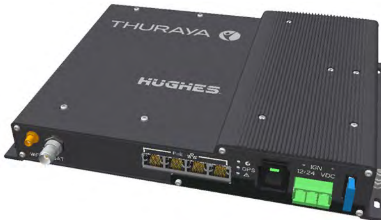
Figure 1-2. Below Decks Unit (BDU)
