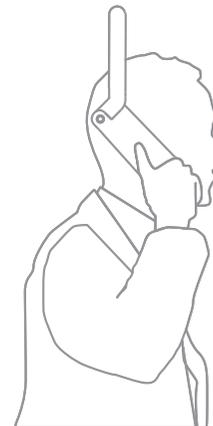
Stand outside with a clear view of the sky with the phone antenna pointing upwards. There must be a clear line of sight between the phone's antenna and the satellite.
